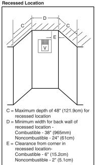
Figure 20 - Minimum Clearances for Vent Terminations
